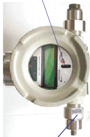
Figure 16 Activating LCD display with magnet.
